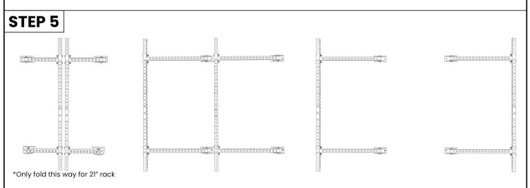
TO FOLD REMOVE PINS, PULL-UP BAR AND J CUPS. LIFT THE UPRIGHT FROM THE BASE AND SWING IT IN THE DIRECTION YOU WANT TO FOLD IN. FOLDING GUIDES ARE AS DISPLAYED ABOVE.
