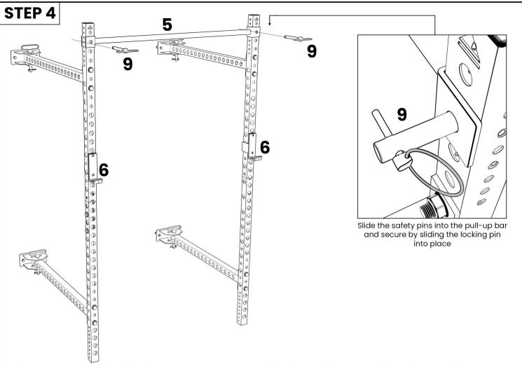
Once assembled with the pull-up bar hold the rack against the wall and you may begin to install the rack to your wall at your own discretion.
