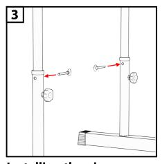
**Installing the pins**For added stability, insert the safety pins into the lower base to secure the upper frame.
