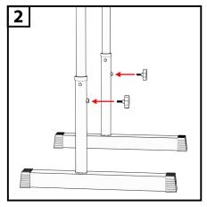
**Installing the knobs**Screw in the adjustment knobs to secure the upper frame in place
