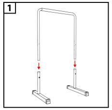
Installing the frame
